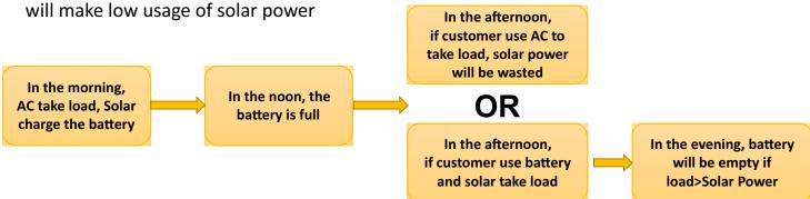
➤ For Sonar Off grid inverter, you can use PV and utility take load and keep battery full at the same time
